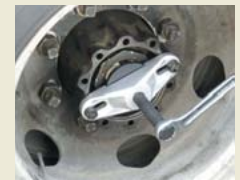
*An off-set wrench (with 27mm width across flat) or a socket with a drive tool (sold separately) is required for operation.
