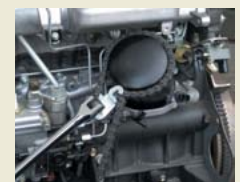
*A 1/2"sq spinner handle or an off-set wrench (with 24mm width across flat) (sold separately) is required for operation.
