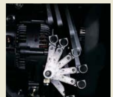
(Photo 3) Fast operation is possible with crank motion.
