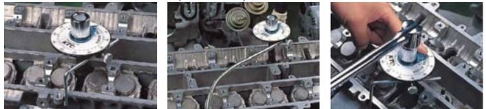
2. Set the angle torque gauge and fix it with the L-stopper or the flexible stopper.
